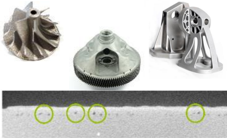
CT - scan highlighting pores/defects
